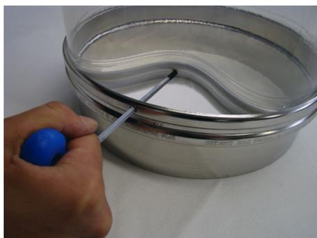
**01.** Insert the removal tool in the opening of the hole and push towards the centre of the fitting.
