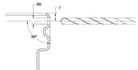
A 6mm hole is drilled in a standard spigot in the position shown above.
