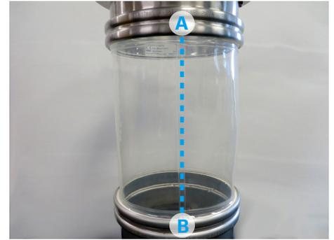
**03.** Snap into the second spigot, ensuring that the welded seam of the connector is straight and that points A and B are directly in line.
