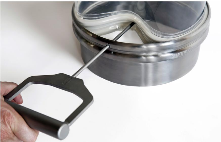
Once a BFM® TR connector is fitted, it is virtually impossible to remove it manually. It is, however, straightforward to remove using a TR Release Tool, which is simply inserted into a 6mm hole in the side of both the upper and lower spigots.
