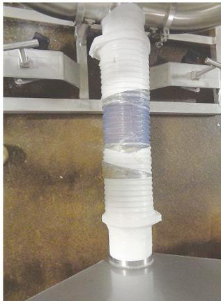
Original connectors were often taped to prevent leakage
