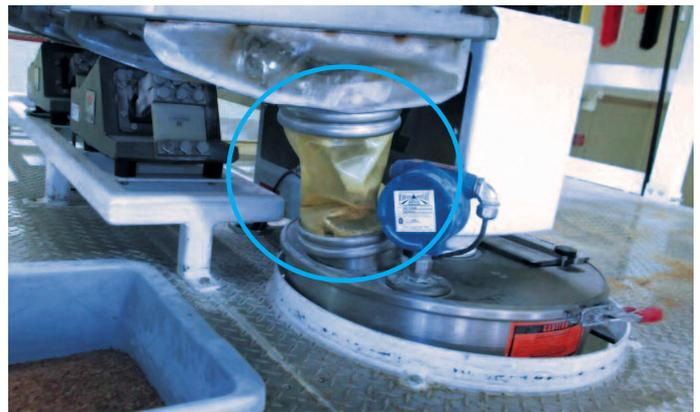
VIBRATORY SCREEN DISCHARGE TO AUGER FEEDER INLET - AFTER
